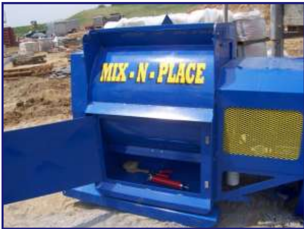
Tool box for storing grease gun, cleaning brush, etc.
